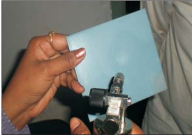
5 Minutes Kept in Gas Torch Flame
