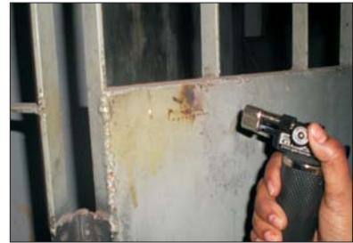
Enamel Paint Starts Burning within 30sec
