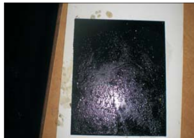
After 30 minutes acid immersion - No affect.
